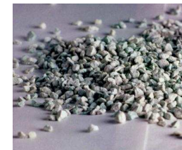
zéolite S_{\text{spé}} \sim 300 \text{ m}^2/\text{g}
