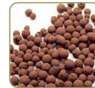
argile expansée S_{\text{spé}} \sim 300 \text{ m}^2/\text{g}
