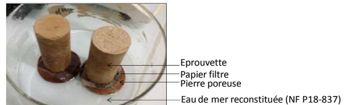
FIGURE 4. DISPOSITIF EXPÉRIMENTAL POUR L'HUMIDIFICATION PAR MONTÉE CAPILLAIRE
