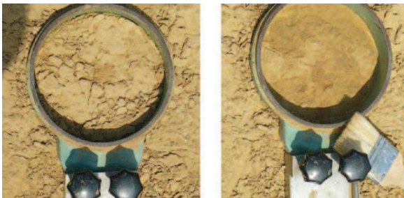
Figure 8: On left the flaky crust which appeared between 28 and 180 days after the construction. On right, this crust is removed using a brush.
